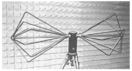
Our biconical-dipole antennas is suitable for measuring radiated emissions as per FCC, EN/CISPR, SAE, MIL-STD and Tempest requirements. They may be supplied with collapsible elements for ease of transport and storage. The elements and the pedestal are made of aluminum to provide a durable,light-weight,corrosion-resis-ta nt antenna.
